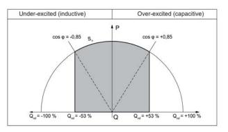
Fig. 4. Possible working area of the inverter. All valid operating points defined by active and reactive power, P and Q, are within the grey area. [5]
