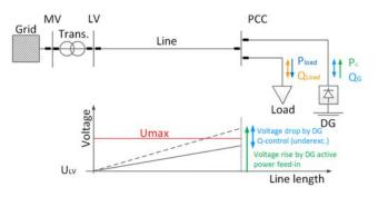
Fig. 1. Impact of active and reactive power on the voltage. [4]
