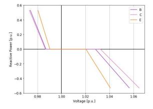
Fig. 8. Parameterised Q(U) characteristic curve of three battery inverters at different positions.
