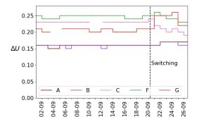
Fig. 12.  $\Delta U$  for all battery systems. On 20 September the grid was switched.
