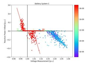
Fig. 14. Reactive power infeed versus the voltage measurement for the battery system C. The colour indicates the time course.
