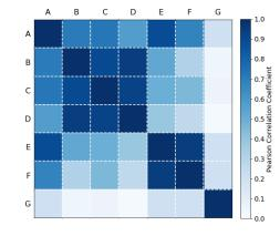
Fig. 10. Correlation of the reactive power infeed of the different battery systems from 1 August to 20 September.
