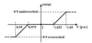
Fig. 4. Reactive control characteristic depending on local voltage.
