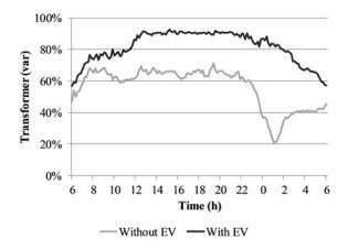
Fig. 9. Transformer load over the course of a weekday for controlled charging and no connected EV's displayed for the 99.97% quantil.
