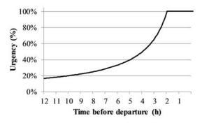
Fig. 1. E.g. change of urgency factor when approaching departure time without charging simultaneously.
