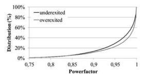
Fig. 6. Power factor distribution for underexited and overexited household loads.
