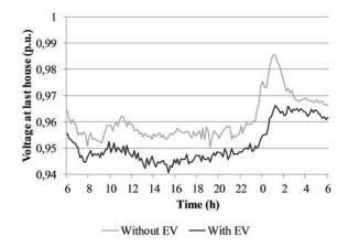
Fig. 10. Local voltage at last household over the course of a weekday for controlled charging and no connected EV's for the 0.27% quantil.
