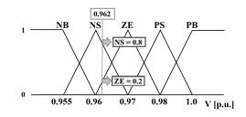
Fig. 2. Evaluation of Fuzzy-Control for local voltage values.
