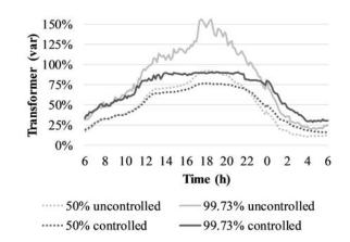
Fig. 7. Transformer load over the course of a weekday for controlled and uncontrolled charging.
