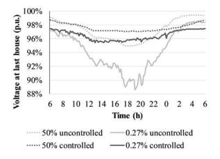
Fig. 8. Local voltage at the last household over the course of a weekday for controlled and uncontrolled charging.
