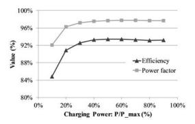
Fig. 5. Charging efficiency and power factor depending on the charging power [8].
