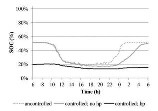
Fig. 11. Minimum SOC over the course of a weekday for controlled charging with and without additional heat pumps and uncontrolled charging.
