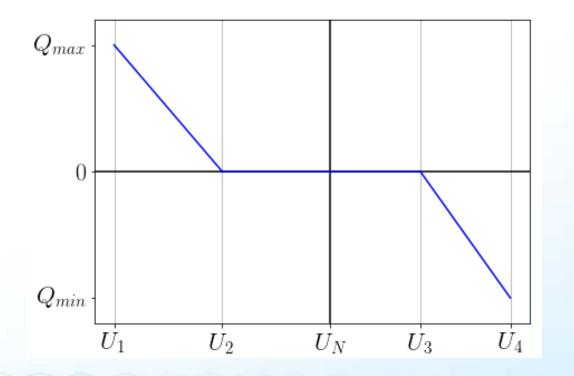
Parameter: $Q_{max}, Q_{min}$ : Max./ min. reactive power $U_N$ : Nominal Voltage $U_{max}, U_{min}$ : Max./ min. measured voltageParameterization: $U_4 = U_{max}$  $U_3 = U_N + 0.5 \cdot (U_{max} - U_N)$  $U_1 = U_{min}$  $U_2 = U_{min} + 0.5 \cdot (U_N - U_{min})$
